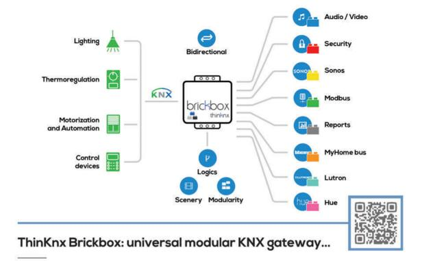
Brickbox is the ThinKnx product line that allows the connection to KNX plant of systems that don't natively support this protocol. Taking advantage of all the functions already integrated in ThinKnx products, through Brickbox it is possible to control, in a bidirectional and fully configurable way, audio sources like Sonos, multimedia systems, alarm devices and systems based on other buses like Modbus, SCS (MyHome), etc.
