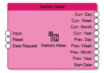
The Statistic Meter reads the numeric value of the **Input** connector and calculates:
