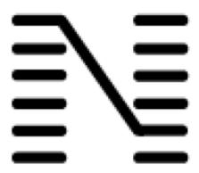
The Logic Matrix, given some inputs determined by the **Number of inputs** property and some outputs determined by the **Number of outputs** property, forwards the value of a selected input to a selected output. The selection of inputs and outputs is decided by the value of two inputs, **Input selector** and **Output selector**.
