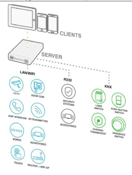
Figure 1: Scheme of a typical integrated installation
