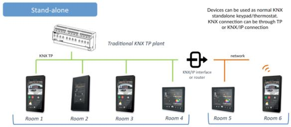
Devices connected over KNX twisted pair
