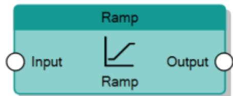
The Ramp node increases or decreases in a linear way the value of the **Output** connector until it reaches the value of the **Input** connector. The linear increment consists of adding (or subtracting) to the **Output** a value represented by the **Step size** property every time interval specified by the **Time step** property.
