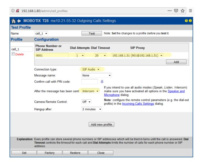
Add the extension 9001 as Phone Number or SIP Address. Under "SIP Proxy", select the option whith the following template "IP\_Thinknx\_Server(9001@IP\_Thinknx\_Server)".
