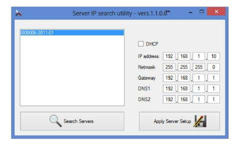
The application program Server manager is installed together with the configurator tool. It searches the network for connected servers and shows the actual IP configuration of each device. After selecting the correct device it is possible to change the IP settings (default configuration is DHCP) and save them pressing the button "Apply Server Setup". It is highly recommended to turn off DHCP and use a static IP address in order to avoid future connection problems.
